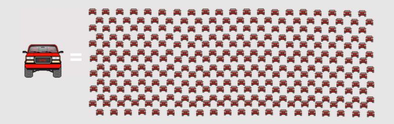
The impact of tampering becomes apparent when you look at the emission increases on a fully deleted vehicle. Testing was conducted without the SCR, DPF, DOC and EGR emission controls NOx increased by approximately 310 times NMHC increased by approximately 1,140 times CO increased by approximately 12 times PM increased by approximately 40 times \*Source: USEPA, Chief Evan Besler, Vehicle and Engine Enforcement Branch; Summit with NJDEP & EPA Region 2
